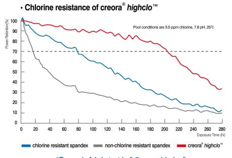
"Dynamic fabric test in 3.5 ppm chlorine"
