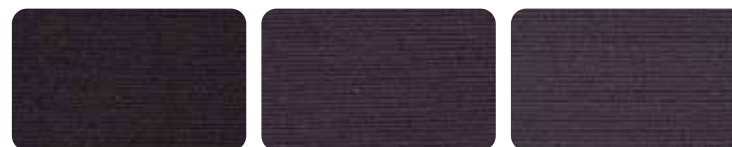
A B C Circular knitting double jersey : Nylon 100/96 + black spandex 70d
